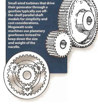
son is that most backyard turbines are direct drive — the generator connects directly to the rotor shaft. So any braking that the generator applies impinges directly on the rotor shaft. (A few such devices employ a gearbox between the rotor shaft and the generator, but the gearbox is typically a simple single-stage parallel-shaft design.)
